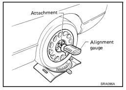
If outside the standard value, adjust with adjusting bolt in front lower link.
