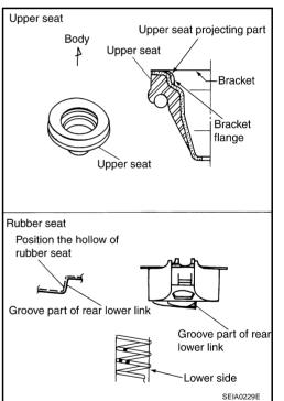
Perform final tightening of rear suspension member and axle installation position (rubber bushing) under unladen conditions with tires on level ground. Check wheel alignment. Refer to <u>RSU-18</u>, "Wheel Alignment (Unladen\*)"
